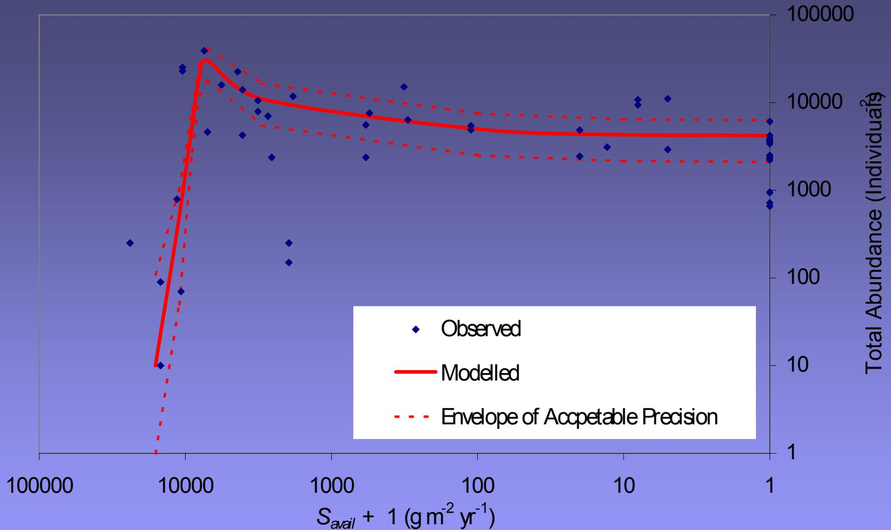
DEPOMOD modelled solids accumulation ( $S_{avail}$ ) plotted against observed total abundance. Envelope of Acceptable precision is shown by the dashed line (68% in EAP,  $n=50$ ).
