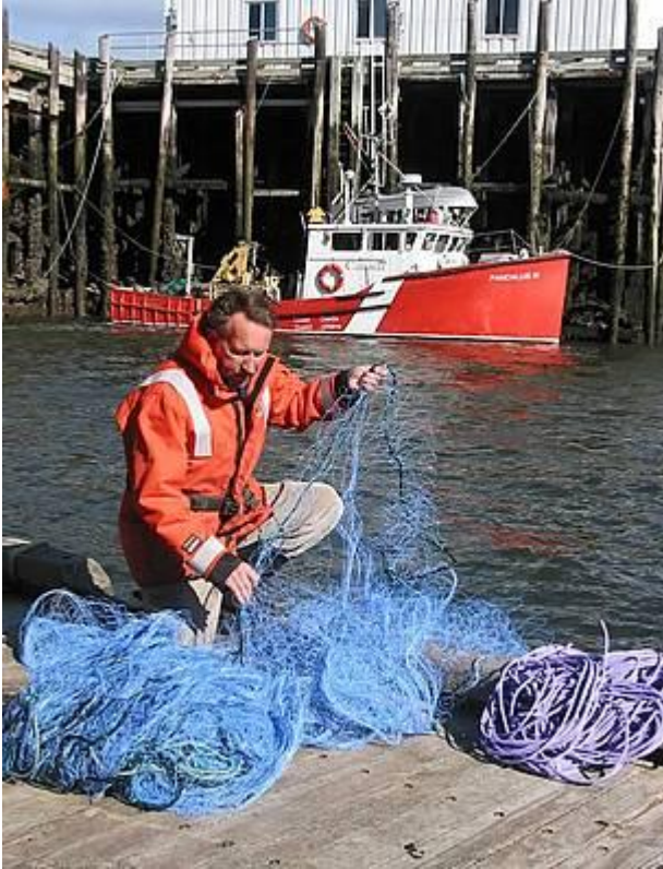
Dr. Ed Trippel at the St. Andrews Biological Station preparing barium sulfate gillnet and weak rope for experimental field trials in the Bay of Fundy, Canada.
